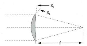
For other forms of simple lenses, the following applies (Note:  $\emptyset$  = power):  $\frac{1}{\text{EFL}} = \emptyset = \frac{1}{2} \left[ \frac{1}{R_1} - \frac{1}{R_2} \right]$
