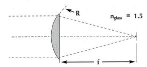
For the plano-convex lens, the focal length equals twice the radius of the convex surface. This is also true for the plano-concave; however, since the radius is negative, this results in a negative focal length: f=2R
