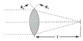
For the double-convex or double-concave lens having equal radii, the focal length will equal the radius:  $R_1=R_2=f$
