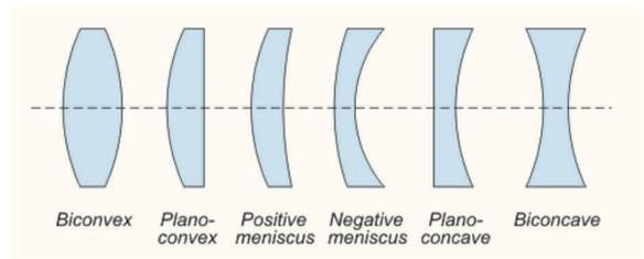
Many of the lens blanks manufactured at AGI are spherical. A spherical surface is described by its radius of curvature (i.e. the radius of the sphere the surface follows). Some commonly used properties of lenses and their calculations for spherical lenses are described below. For more formulas, check out our [simple lens approximations reference chart](#).
