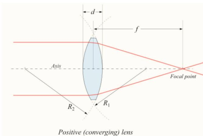
The **focal length** of a lens is the distance over which initially collimated rays are brought to a focus at the focal point. Using the Lensmaker's Equation, focal length can be computed as:
